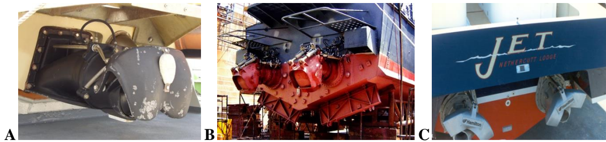
Figure 3.20: The exemplary waterjet drive steering nozzles – sources: A [43], B [44], C [45].
