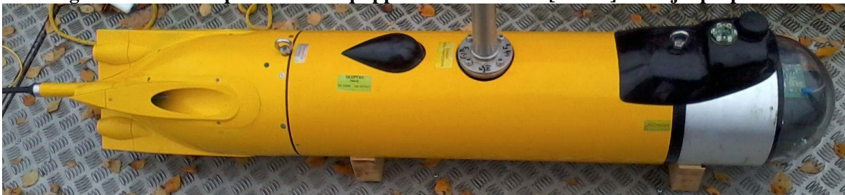
Figure 9.5: The Gluptak vehicle equipped with four WJ50 [50mm] waterjet propulsors.
