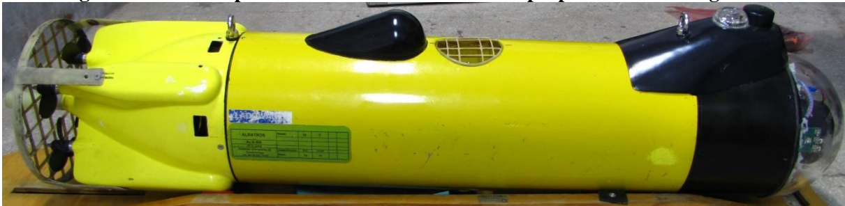
Figure 9.2: The Gluptak vehicle with standard propellers and propellers' guard – SP+G configuration.
