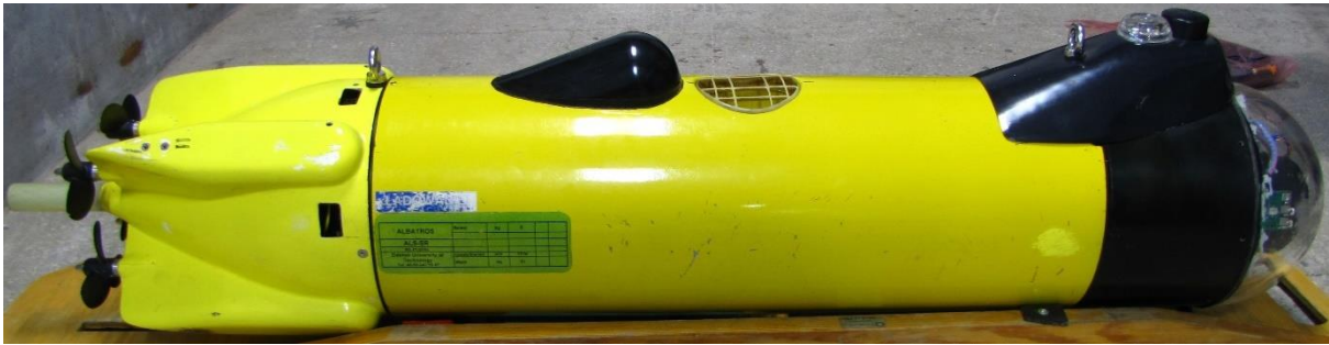
Figure 9.1: The Gluptak vehicle with standard screw propellers – SP configuration.
