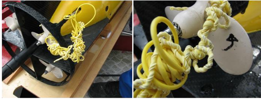
Figure 4.4: The tether entangled in one of the propellers of the GLUPTAK vehicle.
