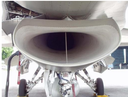
Figure 8.11: F-16 B jet fighter – clearly visible gap between airframe and the engine inlet [115] .
