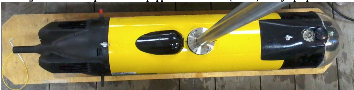
Figure 9.4: The Gluptak vehicle equipped with four G49 [49mm] waterjet propulsors.
