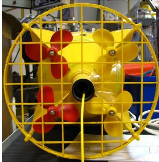
Figure 4.2: The GLUPTAK vehicle with propellers with a mesh-guard configuration – stern view. Arrangement of four screw propeller set. Directivity of the propellers is colour-coded to avoid mistakes during assembly.
