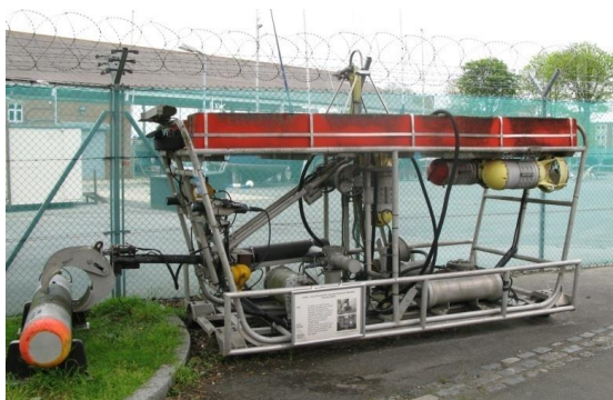
Figure 3.3: The first ROV used by British Royal Navy to recover torpedoes and mines. [5]
